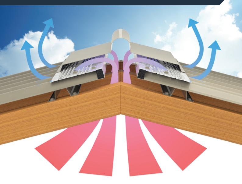
VENT-A-ROOF<sup>®</sup> is a unique passive ridge ventilation system that promotes the circulation of fresh air through roof spaces, ceiling and building spaces in commercial and light industrial buildings, residential homes and most metal sheds.
