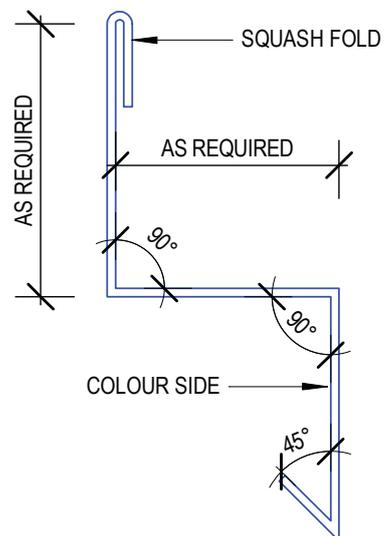
HOR-101 – Z Mould Flashing
