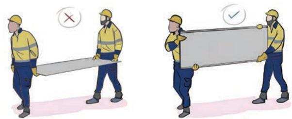
For the handling of heavy panels, it is recommended to use grips (either suction or magnetic grips) to assist in maneuvering and holding the panels in position during installation.
