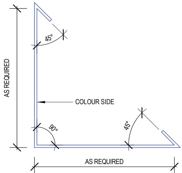
HOR-102 - L Mould Flashing
