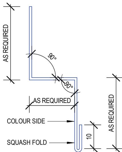
HOR-101 - Z Mould Flashing
