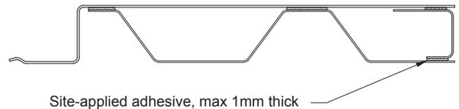
The edge of the trimmed panel will require securing as detailed below. Sealing between the mating surfaces at the exposed leg of the edge trim may be required. If required, the trimmed edge can be concealed with over-flashing.
