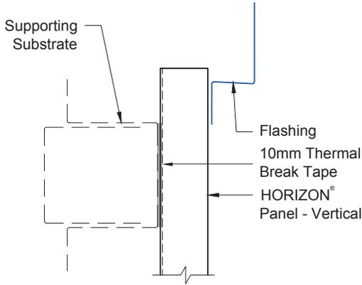
Under-flashing is an alternative approach where the flashing is installed underneath the panel (Figure 4.4-2) or supporting substrate (Figure 4.4-3), for instance, under the battens. Consideration should be given to the potential water flow pathway behind the cladding to ensure no ponding within the profile.
