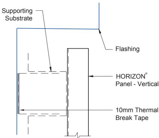
The flashing can be hidden by fastening onto the male leg (Figure 4.4-4) or engaging into the female edge (Figure 4.4-5) of the HORIZON Panel. These flashing details, although more complex, provide a more aesthetically-pleasing effect as they simulate an Expressed Joint.
