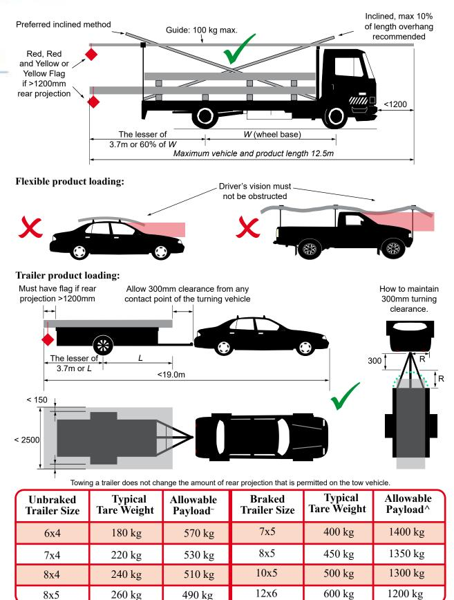
~ Indicative payload of a typical vehicle tow capacity of 750 kg for **unbraked** trailers. ^ Indicative payload of a typical vehicle tow capacity of 1800 kg with a **braked** trailer.
