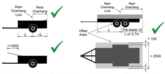
The rear overhang of a trailer must be the lesser of the front load carrying area or body ahead of the centre of the axle group (L) and 3.7 m. Towing a trailer does not change the amount of rear projection that is permitted on the tow vehicle.
