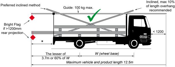
\* Maximum 1200mm for vehicles less than 4.5 tonne GVM in Victoria (provided the rear overhang is less than 3.7m or 60% W).
