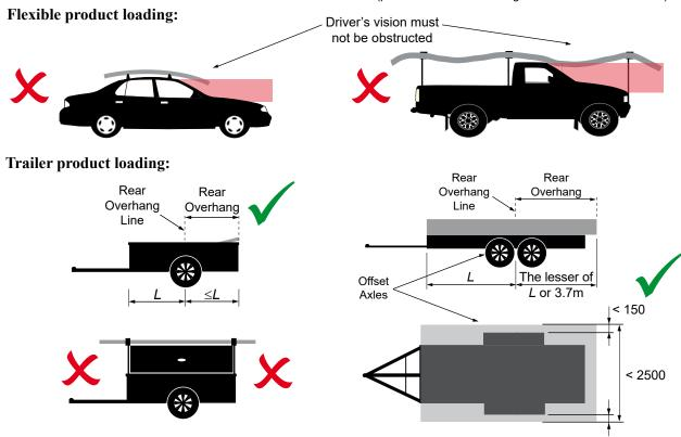
The rear overhang of a trailer must be the lesser of the front load carrying area or body ahead of the centre of the axle group (L) and 3.7m.
