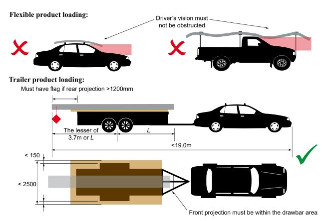
Towing a trailer does not change the amount of rear projection that is permitted on the tow vehicle.
