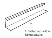
2. Bend Edgeform to required angle.
