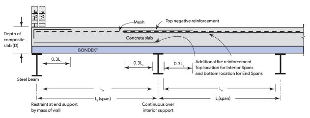
Note: 1/3 top negative reinforcement shall continue all over the span if ratio of live load to total dead load is more than 2.
