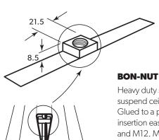
Heavy duty square nut to suspend ceilings or services. Glued to a paper strip it makes insertion easy. Threads: M8, M10 and M12. M6 is available for light loads only (2.7 kN or less).
