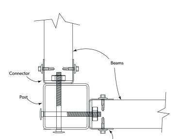
With the framework now in place, double check every dimension against the construction drawing provided and check the diagonals for good measure.
