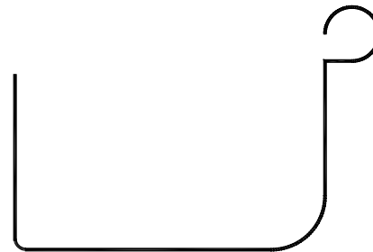
QUAD GUTTER (SECTION)
