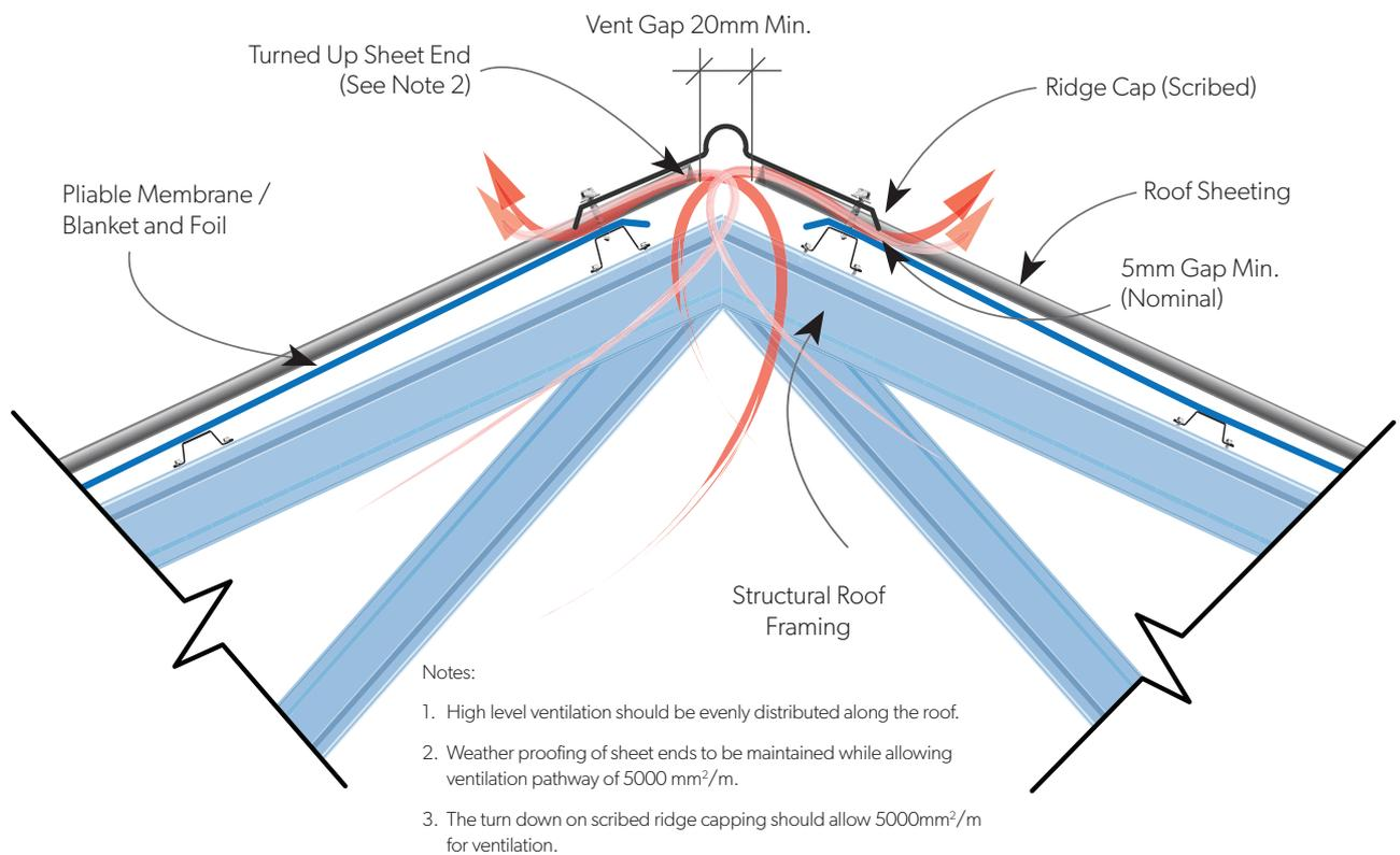
**Figure 4b: High level profile ventilation for trussed roof (10 to 75 degree roof pitch) with no membrane.**
