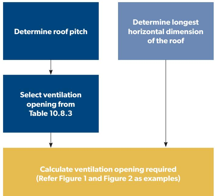
**Figure 1: High level ventilation calculation for a gable roof.**
