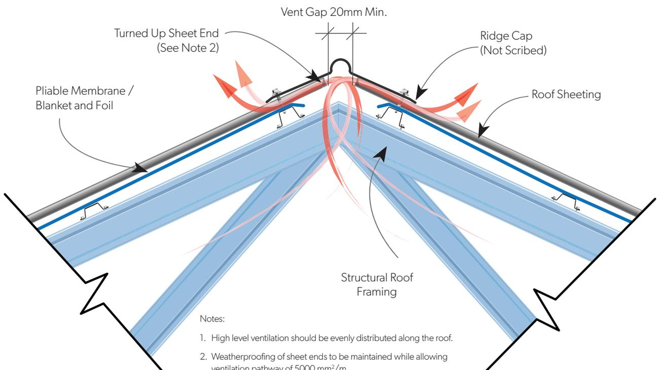
**Figure 3b: High level profile ventilation for trussed roof (10 to 75 degree roof pitch) with no membrane.**
