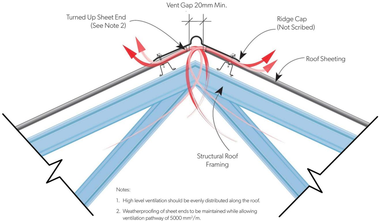
**Figure 4a: High level profile ventilation for trussed roof (10 to 75 degree roof pitch) with membrane cut detail. Wide pan roof sheeting example.**
