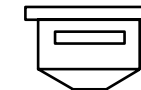
Tapered rainwater heads (downpipe outlet not included) Small: 380 x 175 x 200 mm Large: 450 x 250 x 250 mm Or to your dimensioned drawing.
