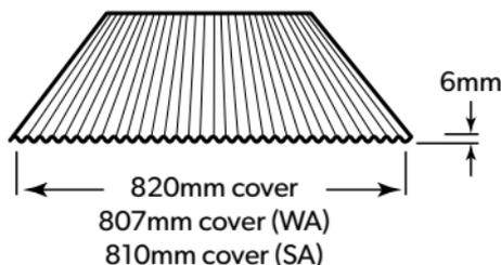
LYSAGHT MINI ORB® is a corrugated sheet with reduced height of corrugation compared to the more traditional LYSAGHT CUSTOM ORB® profile. It is suitable for interior and exterior applications; on straight or curved surfaces; with the corrugations running vertically or horizontally.
