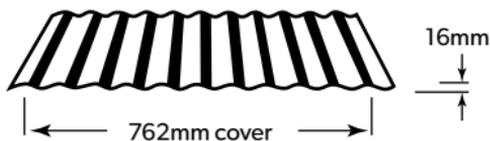
LYSAGHT WALLCLAD® is a lightweight and attractive corrugated walling sheet with the same traditional profile as LYSAGHT CUSTOM ORB®. LYSAGHT WALLCLAD® can be installed either vertically or horizontally for dynamic effects.
