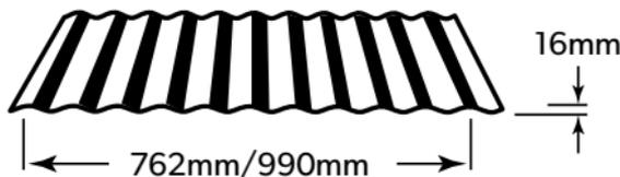
The classic Australian profile is used in traditional as well as modern applications. PERMALITE WAVELINE® is available in 2 widths. Traditional 762mm cover width and our 990mm cover width for greater fixing economy. These cover widths for WAVELINE®, provides a roofing sheet which can also be used effectively on walls.
