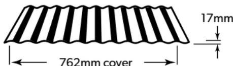
LYSAGHT CUSTOM BLUE ORB® is the corrugated profile perfect for curving, it is the perfect match to harmonise with LYSAGHT CUSTOM ORB®. Roll formed using thicker ductile steel it is used in roofing and walling applications where bull-nosing or curving is required.
