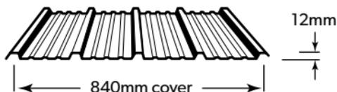
LYSAGHT MULTICLAD® is an attractive trapezoidal multi ribbed profile that is quick and easy to install. It is commonly used in walling for industrial commercial and residential markets.
