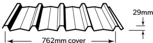
LYSAGHT TRIMDEK® is a subtle square fluted steel cladding profile incorporating fluted pans for strength and long spanning capabilities.
