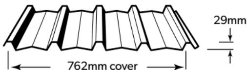
LYSAGHT TRIMWALL® is an attractive, lightweight and versatile steel walling profile designed to complement LYSAGHT TRIMDEK®. TRIMWALL® allows long spans for quick installation.
