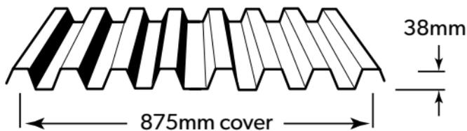
PERMALITE LT7® is the ultimate in cladding flexibility. The versatility of this profile is due to its strength, water carrying capacity, fixing economy and eave closure features. It is widely used for roofing and can be reversed for a bold wall effect.
