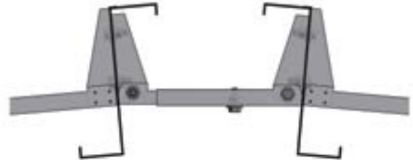
FIGURE 6.1.1-5: MAX-BRIDGE™ ridge member installation
