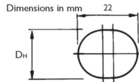
BlueScope Lysaght standard elongated punched hole. Holes equally spaced above and below centre line.
