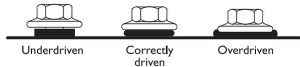
**Figure 4.7: Avoid overtightening screws**
