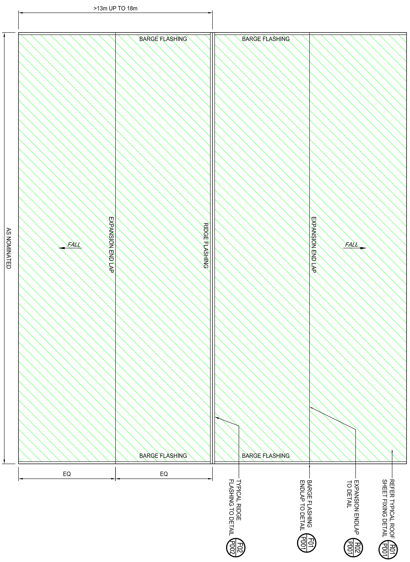
1 TYPICAL ROOF SHEET LAYOUT - ROOF SPAN > 13M AND UP TO 18M PLAN SCALE 1:200
